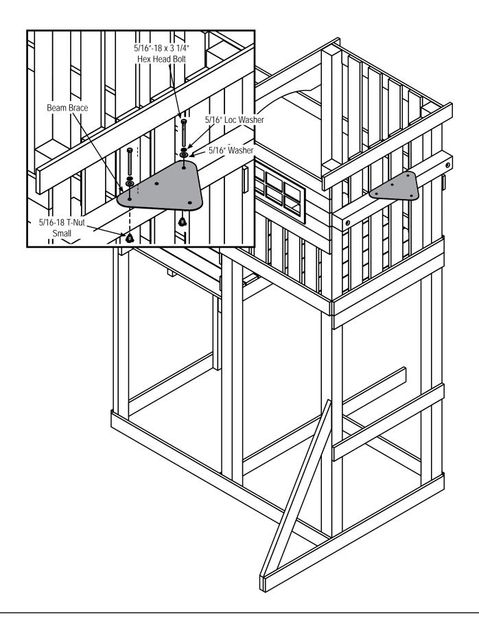
1. Install Swing Beam Brace as shown.
