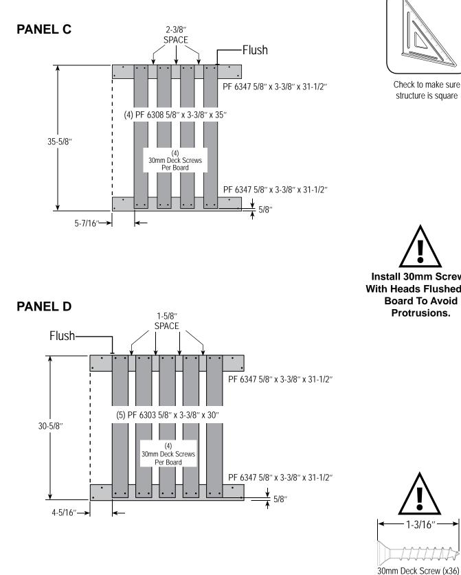
**Install 30mm Screws** With Heads Flushed To **Board To Avoid Protrusions.**
