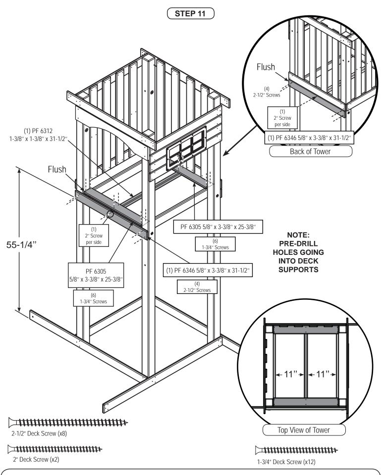
1. Attach Deck Boards and Deck Support Boards as shown.
