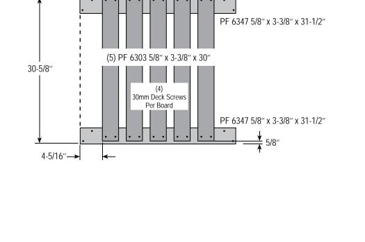
1. Assemble Panel C and Panel D as shown. 2. Mark panels C and D.
