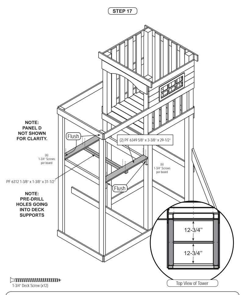
1. Attach Deck Boards and Deck Support Board as shown.
