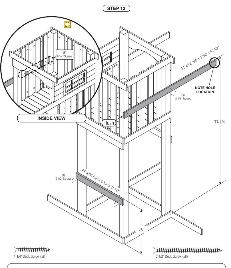
Attach Barrier Support Board and Safety Board as shown.
