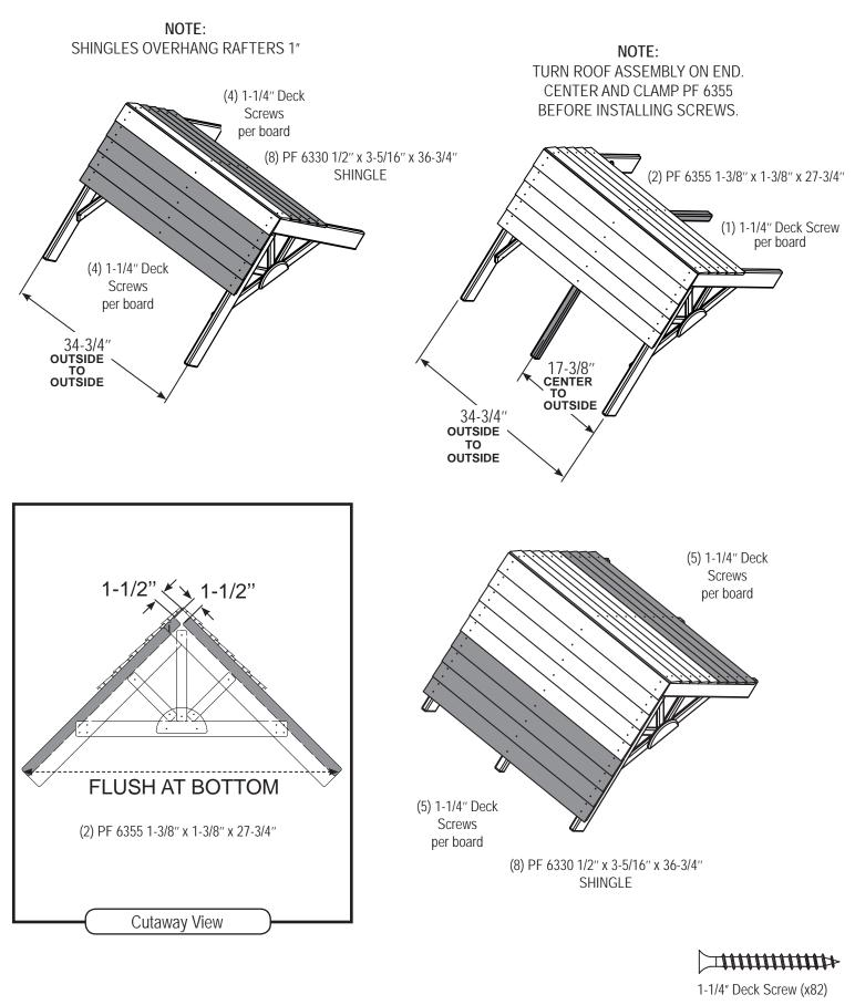
1. Complete Roof Assembly as shown.
