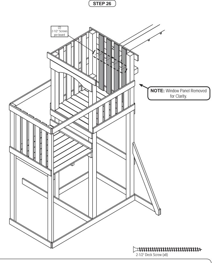
1. Secure Barrier Boards to Swing Beam Support as shown.
