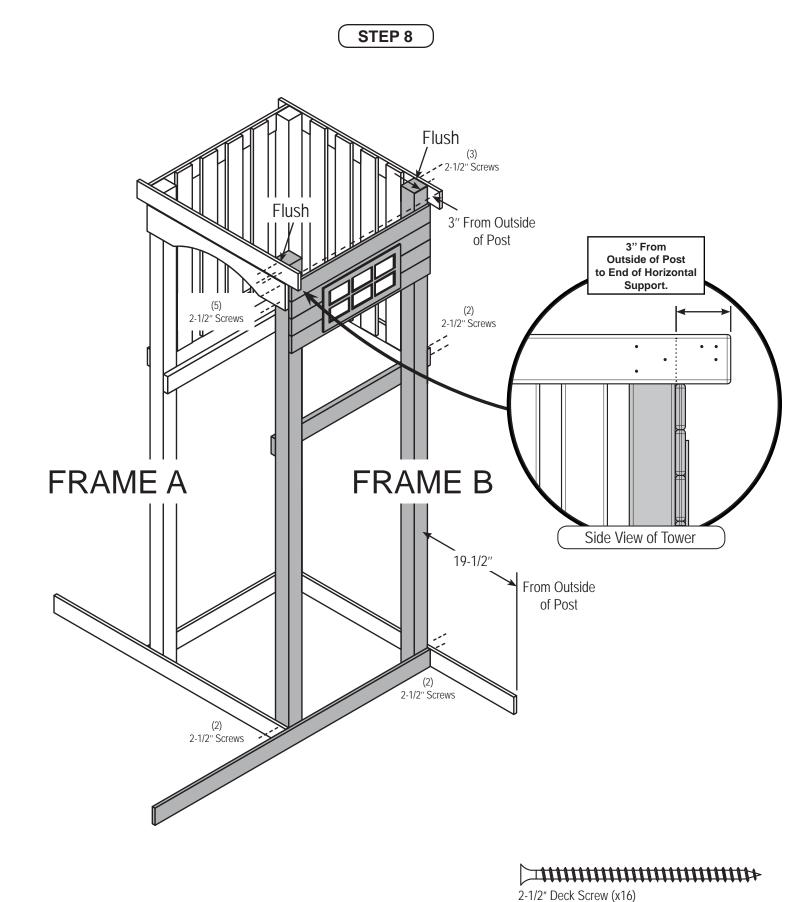
1. Attach Frame B to Frame A as shown.
