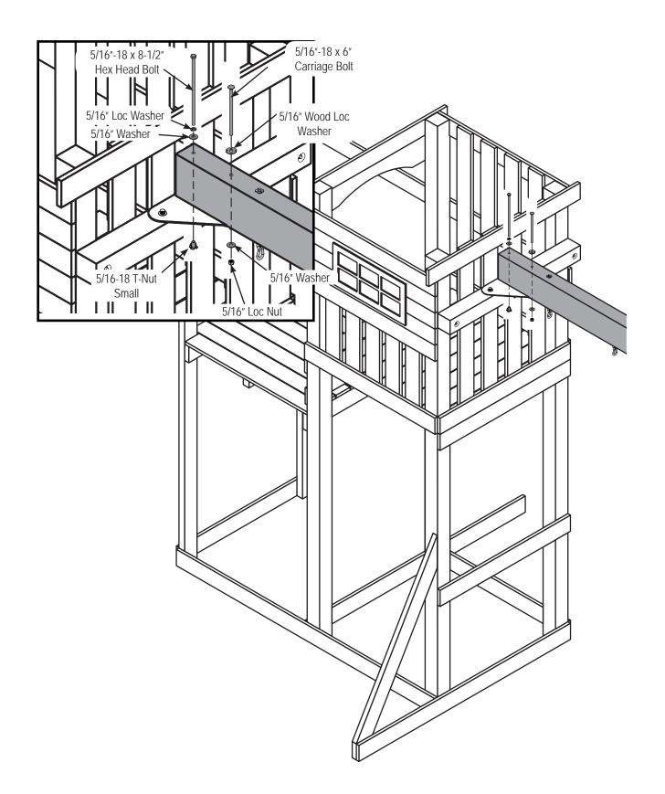
1. Install Swing Beam as shown.
